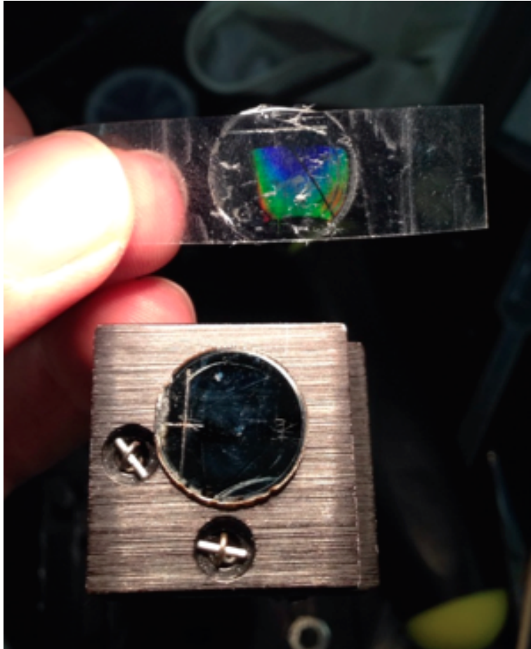
Figure 3.2 Pealed polymere film via double sided tape
